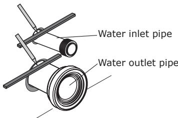
**B:** Insert the pipes into the toilet until they could not move forward; mark cross lines between pipe and toilet back side level.
