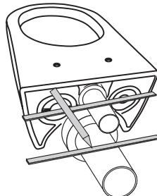
**C:** Cut off the connecting pipe; the cut length should be the sum length of lines in a) & b) and the length showing in the below figure.
