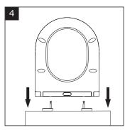
Before attaching the seat, move mounting bases so posts align with holes in the back of the seat. Once aligned, carefully lower the seat (holes) onto the mounting post.
