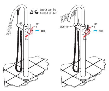
Turn on the tap, turn the handle according to the marks to adjust the temperature.
