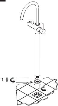
Unfasten the fixing nut by wrench S1.5mm, take off the nut from the body.
